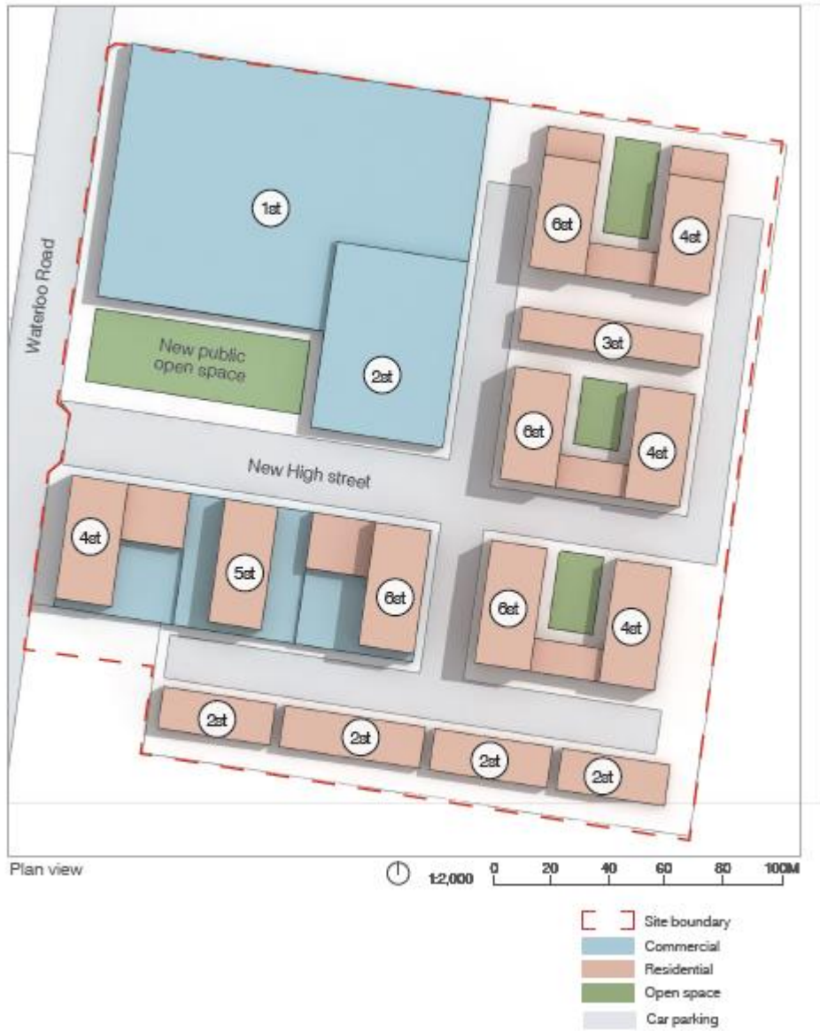
Figure 29 Preferred master plan scenario based on commercial/retail FSR of 0.35:1 and residential FSR of 0.65:1 (source: Architectus – Urban Design Peer Review)
